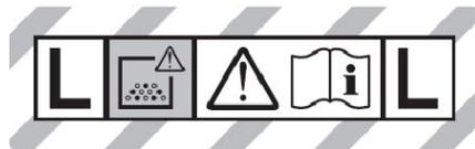
Class L dust extractors are suitable to extract dry, non-combustible dusts with workplace limit values of > 1 mg/m<sup>3</sup>.
