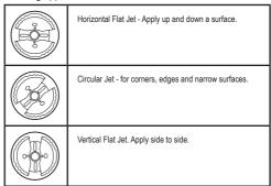
There are three spray patterns to choose from. They are marked as 1, 2 and 3 on the pattern select label located on the top of the sprayer (fig. H)
