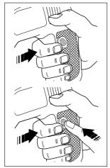
To switch your drill on, depress the variable speed on/off switch. Your drill stops when the switch is released. If continuous operation is required, depress the lockon button while the variable speed on/off switch is depressed. To stop your drill
