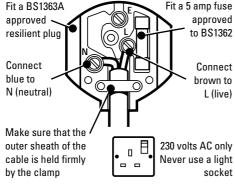
• Before replacing the top cover of the plug ensure that the cable restraint is holding the outer sheath of the cable firmly and that the two leads are correctly
