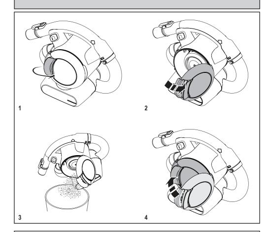
In order to keep the suction force optimised, the filters must be cleared regularly during use. 为了达到最佳吸尘力, 使用过程中必须定期清洁过滤器。
