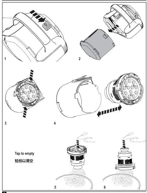
Re-assemble after cleaning the filter or continue to wash.
